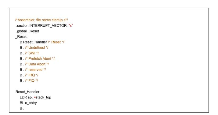
You will compile this using arm-none-eabi-as -mcpu=arm926ej-s -g startup.s -o startup.o . Now you need to link both the files. So you will need a linker.
